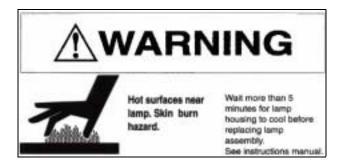
Hot surface near lamp. Skin burn hazard. Wait more than 5 minutes for lamp housing to cool before replacing lamp assembly. See instruction manual.
